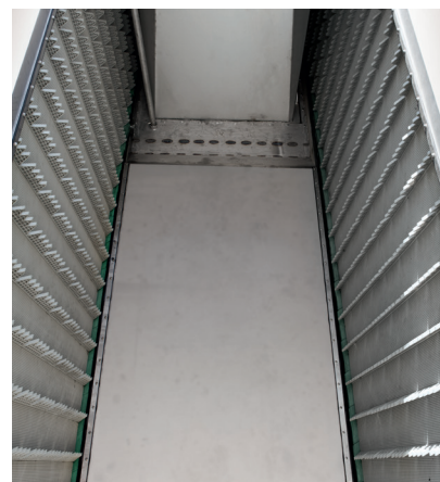
Perforated Plate Version with Lifters.
